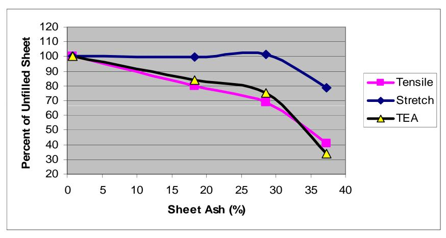
Tensile and TEA show the same trend. Stretch was surprisingly unaffected by sheet ash up to almost 30% filler content. Stretch-to-rupture at press consistency was ~2x that of dry paper.
