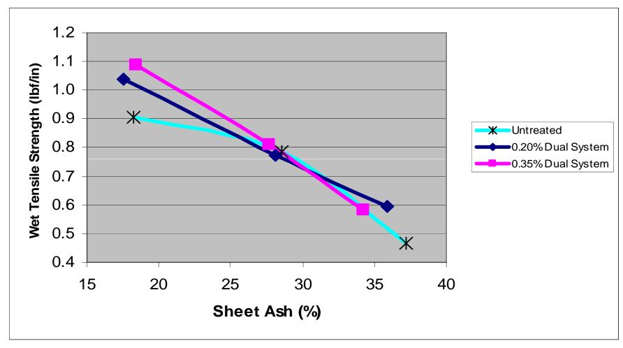
Application of a dual cationic / anionic polyacrylamide strength resin system appeared to have some positive effect upon tensile strength at lower filler content. There was no effect at 28-35% sheet ash.
