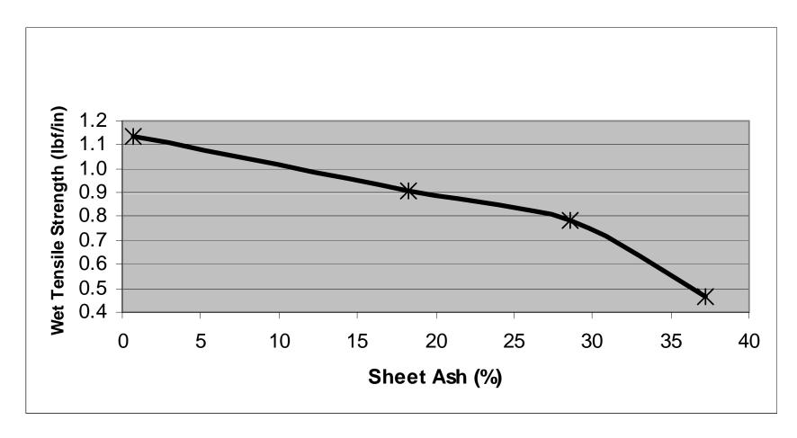
Surprisingly modest drop of about 30% between 0 and 28% sheet ash. Steeper decline thereafter. Limitation: These are non-directional handsheets. Absolute MD strength on a paper machine would be higher at this basis weight.
