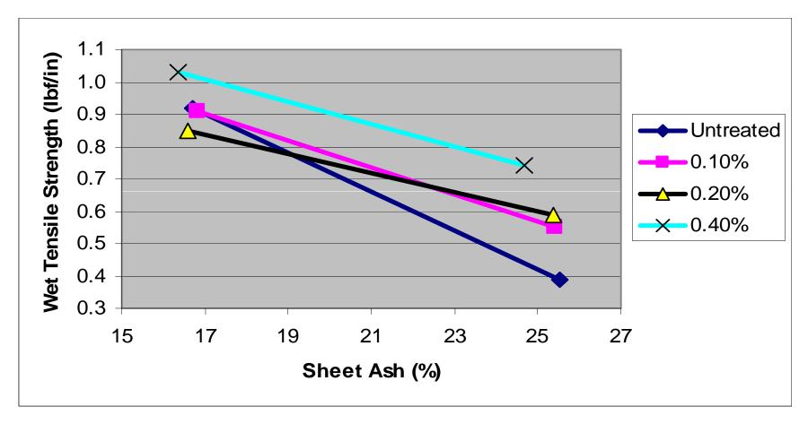
Application of novel amphoteric polymer Hercobond ® HA5305 mitigated twothirds of the tensile loss due to increasing filler content at the highest dosage. The untreated tensile loss was greater than observed in previous experiments.
