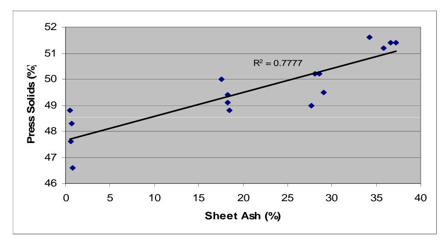
How well were press solids controlled in the previous experiment? Press solids increase with higher sheet ash, and scatter decreases. Increased solids could be partially responsible for lower magnitude impact than expected.
